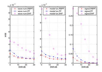
**Fig. 2.** RMSE versus different SNRs for wave numbers (left), modal functions (center) and signal field (right)
