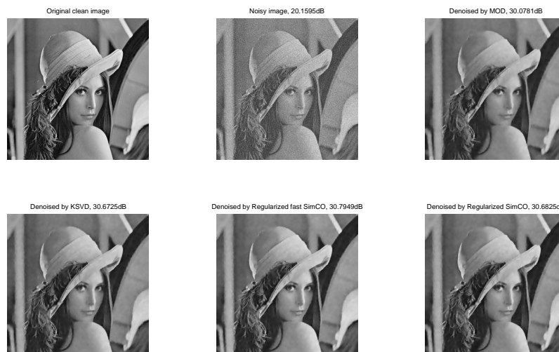
FIGURE 3. Image denoising examples using the fast SimCO compared with other baseline algorithms. PSNR values in dB are given in the sub-figure titles.
