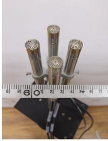
**Fig. 2.** The uniform circular sensor array used in the experiments, with an array radius of 0.02 m.
