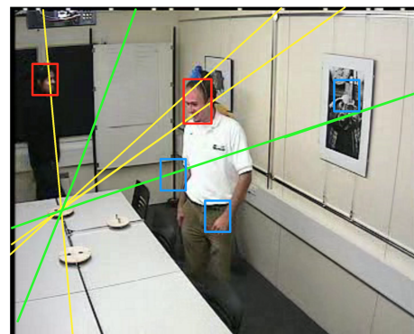
Fig. 10. The clutter at frame 660 of Sequence 45. The face detection, DOA lines, visual clutters, and the audio clutters are shown in the red boxes, yellow lines, blue boxes and green lines, respectively.
