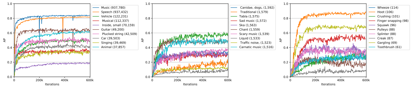
Fig. 3. Class-wise AP of sound events with the CNN14 system. The number inside parentheses indicates the number of training clips. The left, middle, right columns show the AP of sound classes with the number of training clips ranked the 1st to 10th, 250th to 260th and 517th to 527th in the training set of AudioSet.
