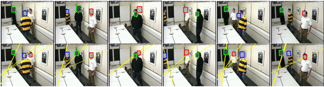
Fig. 7. Sequence 45 camera #3: three speakers with occlusions. The first and second row show the tracking results of the V-SMC-PHD and the proposed AV-SMC-PHD filter, respectively.
