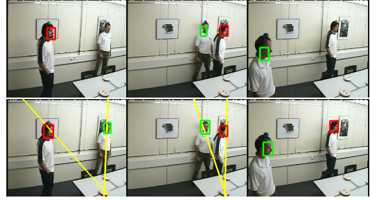
Fig. 3. Sequence 24 (camera #1): Two speakers with occlusions. The first row shows the results of the V-SMC-PHD filter and the second row shows tracking results of our proposed AV-SMC-PHD filter.
