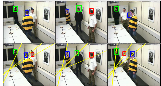
Fig. 5. Sequence 45 (camera #3): Three speakers with occlusions. V-SMC-PHD performance is shown in the first row, and AV-SMC-PHD shows better performance in the second.
