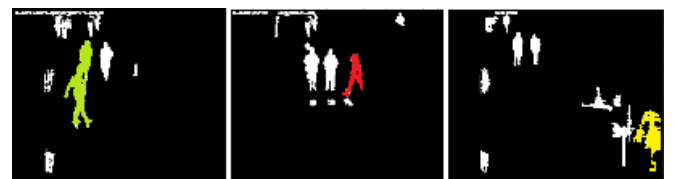
Fig. 2: Background subtraction results for three frames in the sequence, where the green part in the first figure shows the occlusion of two human targets, which may cause miss detection; the red part in the second figure shows the appearance of another human target and the yellow part in the third figure shows the disappearance of a human target; as shown in the figure, there are noises in the background subtraction results, including the patches noises and salt and pepper noise, which may cause false alarm in the multiple tracking work.
