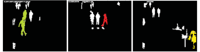
Fig. 2. Background subtraction results for three frames in the sequence, where the green part in the first figure shows the occlusion of two human targets, which may cause miss detection; the red part in the second figure shows the appearance of another human target and the yellow part in the third figure shows the disappearance of a human target; as shown in the figure, there are noises in the background subtraction results, including the patches of noises and salt and pepper noise, which may cause false alarm in the multiple tracking work.
