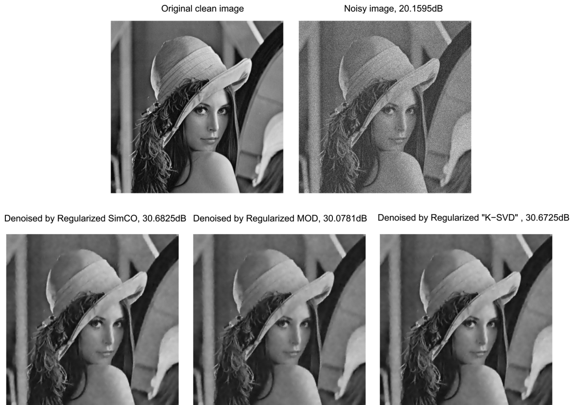
Fig. 4. Example of the image denoising using dictionary learning. PSNR values in dB are given in sub-figure titles.
