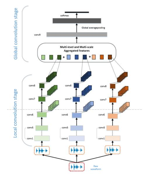
Fig. 1. The overall framework of the multi-channel deep convolutional neural networks environmental sound classification system
