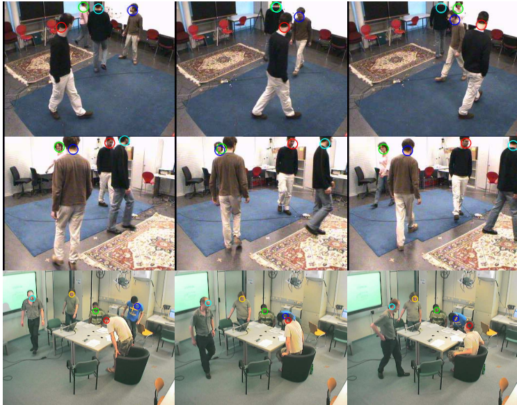
Fig. 15. Multiple person tracking using adaptive identity models. The images in the first two rows are from the EPFL dataset the bottom rows is a sequence from the CLEAR dataset.
