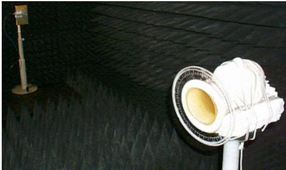
Figure 5-4 Photograph showing the phantom set up on a platform in the anechoic chamber
