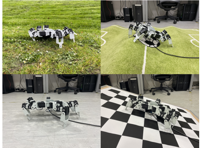
Fig. 1: Terrain aware hexapod robot using motor feedback to determine terrain type and adjust its walking policy accordingly
