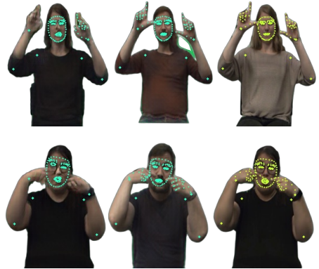
Fig. 7: Qualitative comparison of the pose estimation on the synthesised images of signers. The keypoint estimation is highlighted in colors on top of the image. KEY – left: AnonySign; middle: PENet (ours); right: ground-truth.
