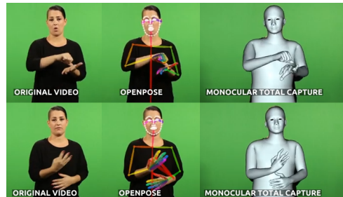
Fig. 1: Figure showing OpenPose failure for hand-to-hand interaction and associated incorrectly reconstructed mesh for Monocular Total Capture.
