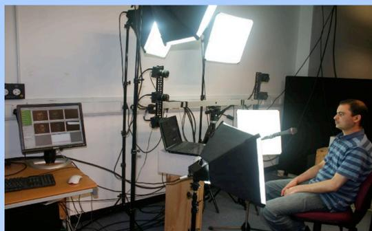
Figure 2. Face capture rig in lab with lighting.
