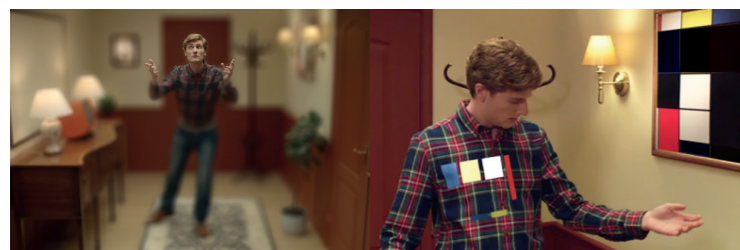
Figure 3: Examples demonstrating digital refocusing (left) and scene augmentation using computer-generated assets (right). In both cases, depth information (in this case captured using an additional depth sensor) is used to facilitate the generation of visual effects and increase creative control. Images produced as part of the EU FP7 project SCENE
