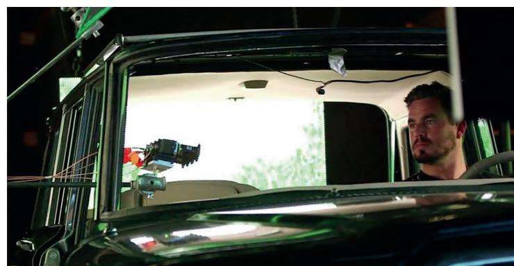
Figure 4: Four-camera rig used by MPC to capture Goosebumps VR demo
