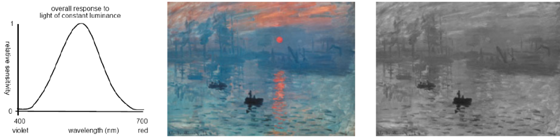
Figure 2.5: Greyscale conversion. Left: The human eye’s combined response (weighted sum of cone responses) to light of increasing wavelength but constant intensity. The perceived luminosity of the light changes as a function of wavelength. Right: A painting (Impressionist Sunrise by Monet) in colour and greyscale; note the isoluminant colours used to paint the sun against the sky.
