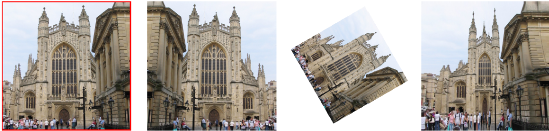
Figure 3.1: Various geometric transformations applied to an image. The results were achieved using two rigid body transformations (reflection, and a combined rotation and scaling) and a non-rigid transformation (pin-cushion distortion). Note that only rigid body transformations can be realised using matrix multiplication.
