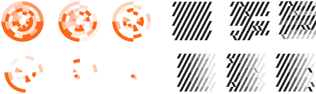
Fig. 6. Developed visualisations deployed in TAPESTRY. Left: Pie communicates interpersonal trust e.g. to help users determine whether to trust an unknown business or service online. Concentric rings of the pie correspond to different granularities of time, and shading is used to communicate coherence and volume of activity within the time period corresponding to each segment. Right: Slash communicates introspective trust e.g. to help users determine if their social media account has been compromised. Each slash corresponds to a period of time, with backslashes indicating anomalous (outlier) TE during that period. Shading is used to communicate volume of TE during that period, as with ‘pie’. Six instances of the visualisations are displayed ranging from complete and coherent, to sparse TE over the time period requested by the verifier.
