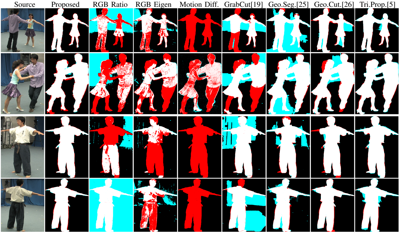
Fig. 2. Multi-view segmentation results for SALSA (upper) and KARATE (lower). Red: under-detected vs. groundtruth. Blue: over-detected vs. groundtruth.
