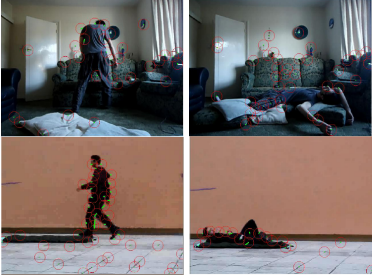
Figure 2. Evaluation dataset: examples of falls present with our two 100 video datasets captured in cluttered and uncluttered conditions. Red circles indicate features; green lines indicate the feature trajectories.
