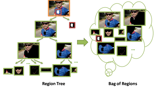
Fig. 2. The “bag of regions” representation of a “biker” example. Regions are collected from all nodes of a region tree generated by [6], ranging in various levels of details.
