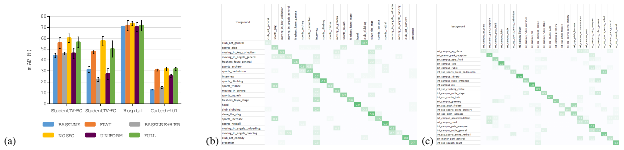
Figure 5: (a) Accuracy (mAP) of the proposed system over three datasets: ‘StudentTV’, ‘Hospital’, ‘Caltech-101’. Refer to Sec. 4.2 for meaning of abbreviations which relate to system configurations. Confusion matrices summarising per-class performance of the proposed system over the foreground and background classes of the ‘StudentTV’ dataset.
