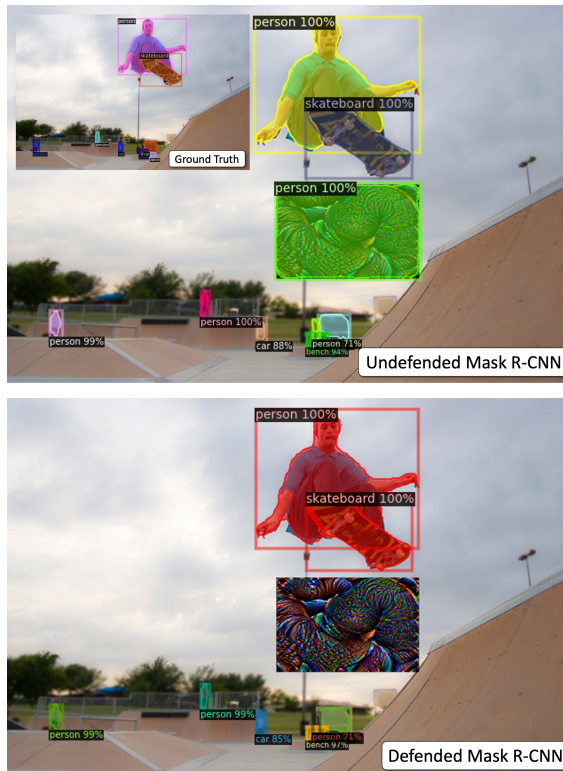
Figure 1. Defending a segmentation network (Mask R-CNN) against an adversarial patch attack introducing a spurious person detection. An undefended Mask R-CNN (top) detects the patch as ‘person’, whereas our defended Mask R-CNN (bottom) ignores the patch and predicts the same as the ground truth (inset).
