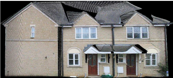
Fig. 9. An example of raw output from an RTcam. Object parts that were obscured in the source photos appear as holes, which are filled-in using by growing surrounding texture into them. Anti-aliasing takes the non-uniform distribution of points into account, as explained in the text.
