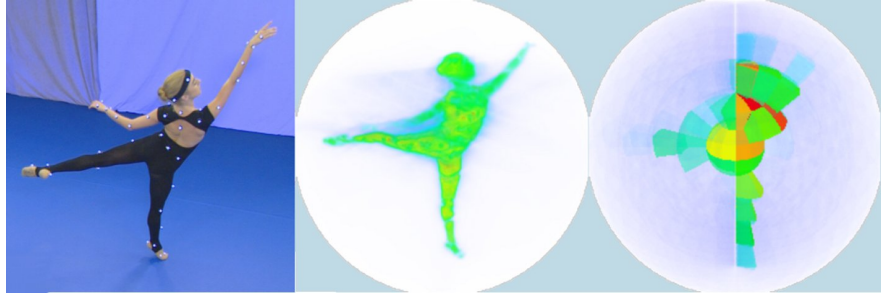
Fig. 6 Visualisation of a spherical histogram computed from a character volume. Multiple video views (left) are combined to produce a volumetric estimate of the character (middle) which is quantized into a spherical (long-lat) representation at multiple radii from the volume centroid.
