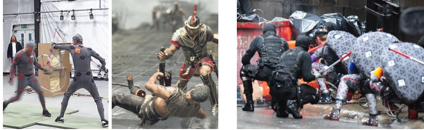
Fig. 1 Performance capture technologies. Left: Vicon IR based system being used to pre-visualize character performance in real-time within the UNREAL Games engine (EPIC). Right: Industrial Light and Magic's fractal suit enabling visual light based tracking outdoors.
