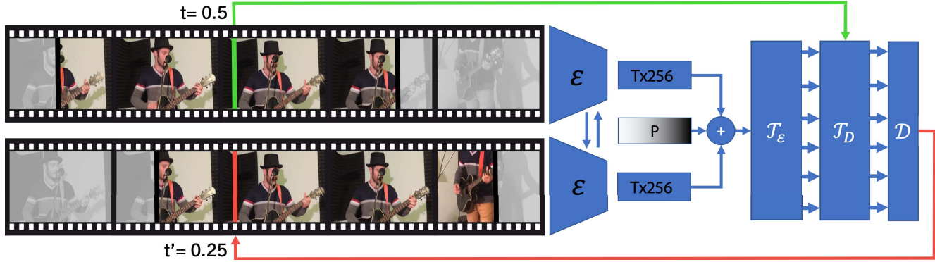
Figure 2. Architecture diagram of the proposed alignment transformer \mathcal{T} . Sequences of robust fingerprints are encoded using \varepsilon(\cdot) [6] from the query V and candidate videos V' . Together with a positional encoding, they are fed into a transformer encoder \mathcal{T}_E . Given query times t , the decoder transformer \mathcal{T}_D provides an output, which is interpreted by an MLP D to match query times with corresponding times t' .
