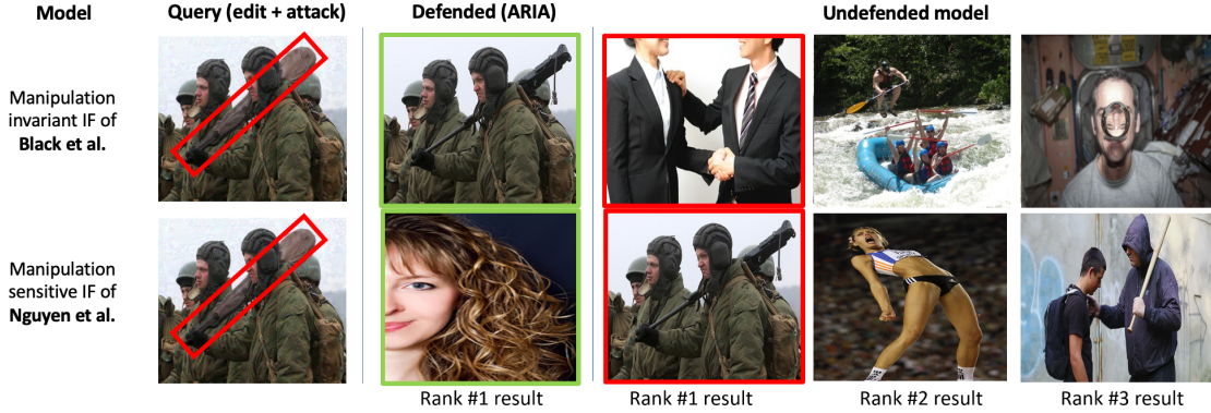
Figure 2. Attacks on image fingerprinting (IF) models. Visualization of untargeted adversarial examples of size \varepsilon_\infty = 8/255 on two IF approaches with complementary goals. Upper: a model seeking to match an original image, invariant to any editorial change in the query [6]. Lower: a model seeking to avoid matching an edited query to the original [45]. In both cases it is possible to attack the model to defeat the goal, and in both cases ARIA defends it successfully.
