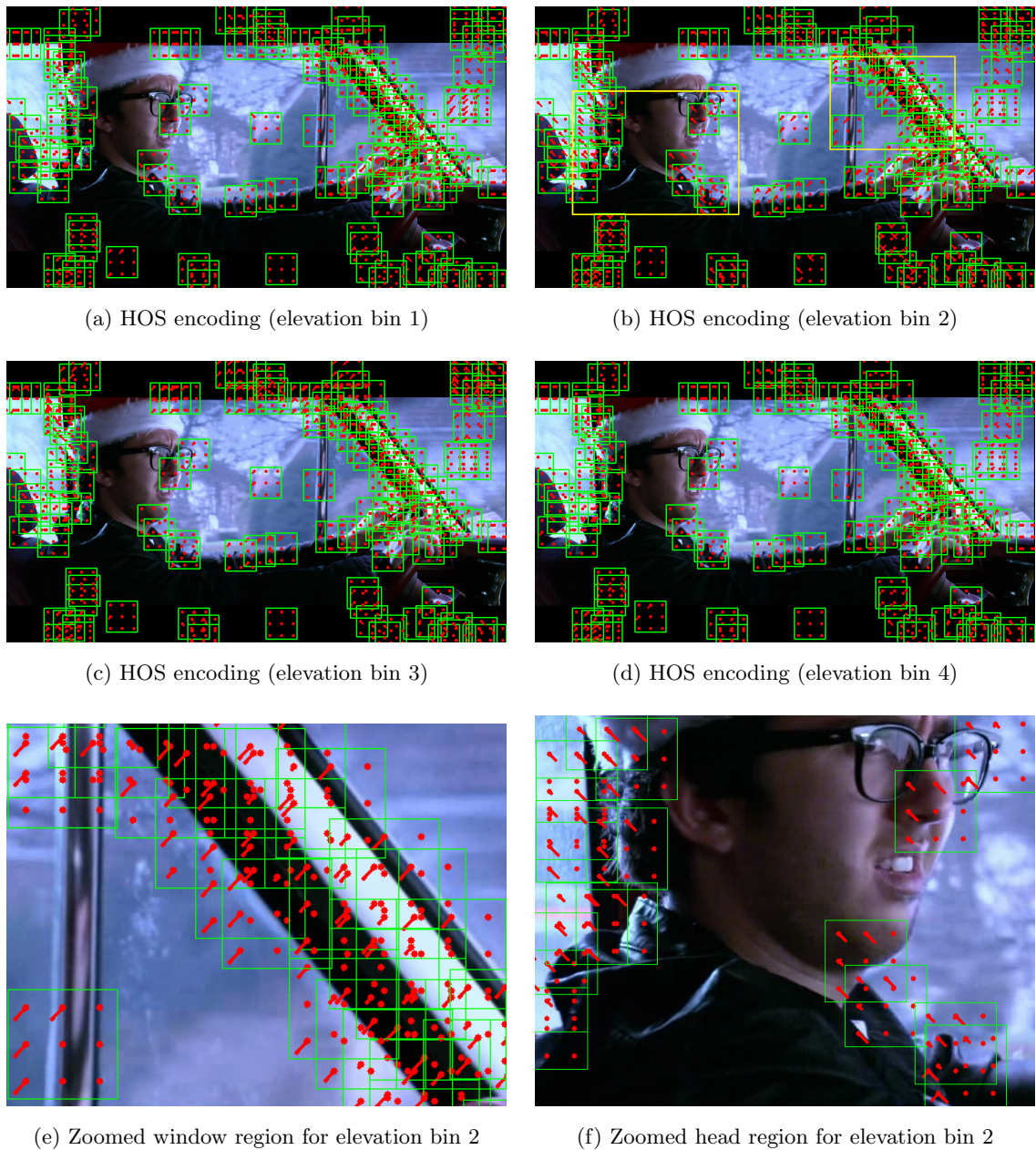
Figure 6.5: HOS encoding for Hollywood 3D Drive example. A large number interest points have been detected, with some overlaps in the local features. Green squares represent blocks, with each red dot being the centre of a cell. Images 6.5e and 6.5f show zoomed regions of interest, indicated by yellow boxes in the original image.
