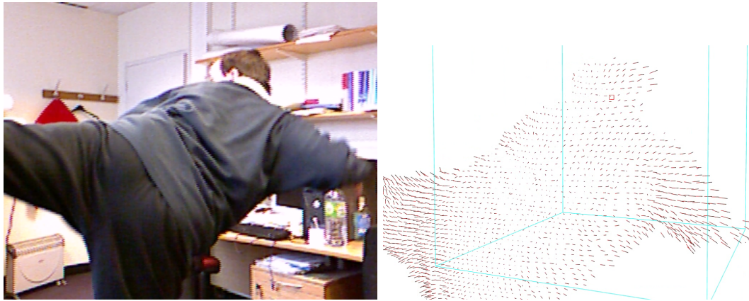
Figure 1.3: An estimated 3D motion field (right), from a sequence of a person performing a kicking action (left). Motion vectors move from the red to purple vertices.
