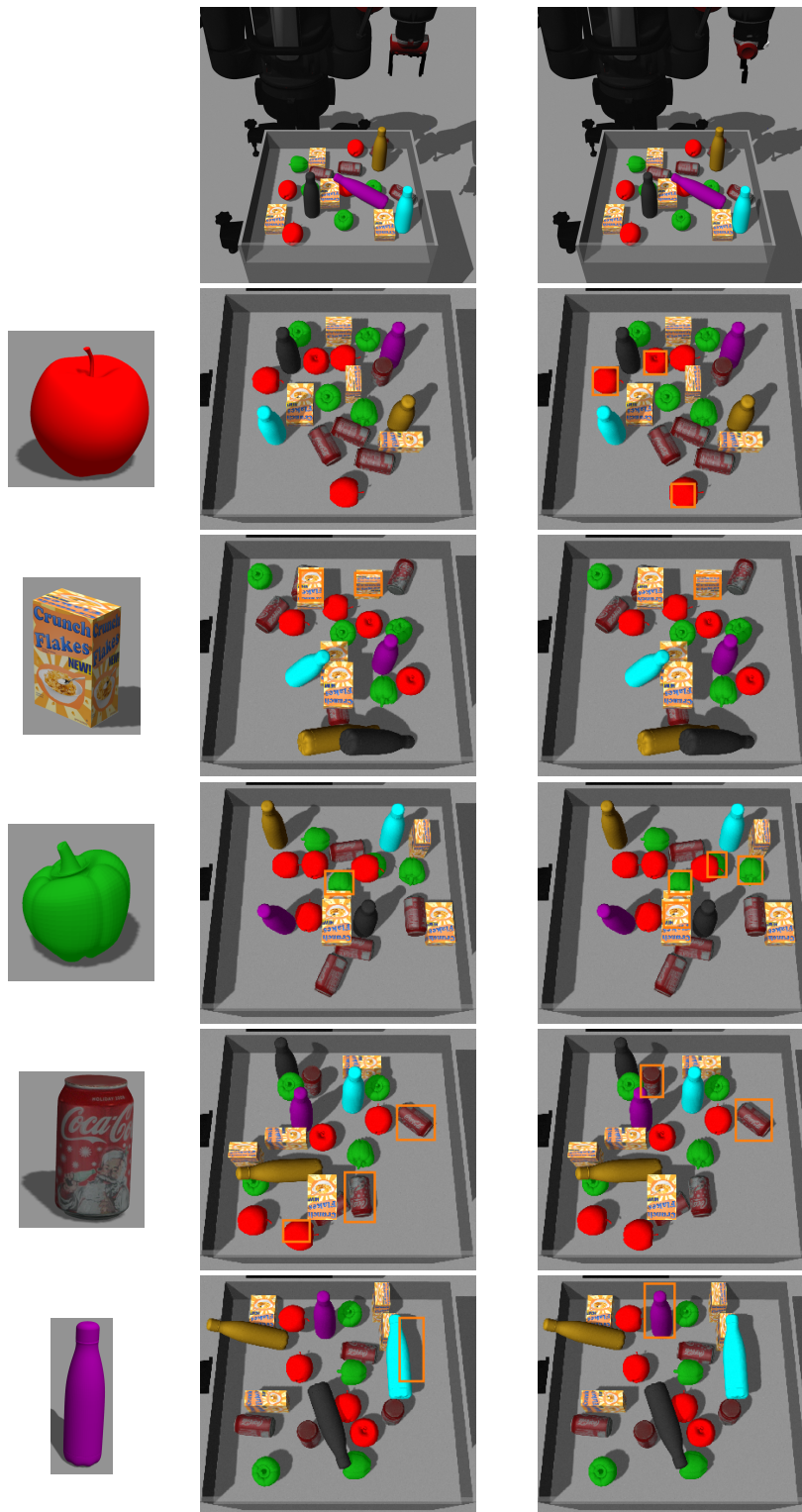
Figure 6.12: Examples of ROD detections with different policies - the first policy uses a policy with the gripper parallel to the the y-axis of the robot, the second policy uses a policy with the gripper parallel to the x-axis of the robot - gripper orientation can be seen in the first row. The conditioning object is shown in the first column.
