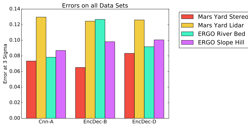
Figure 3.22: 3 sigma error averaged across all model scales, shown for each training dataset and three model topologies.
