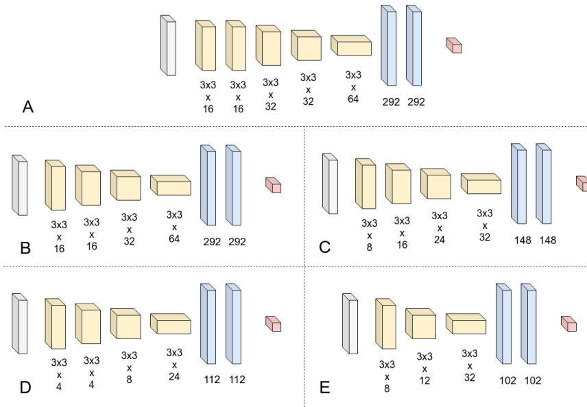
Figure 3.3: High level description of the five CNN models evaluated in our AHS publication [22]. Detailed descriptions of these models can be found in Appendix A
