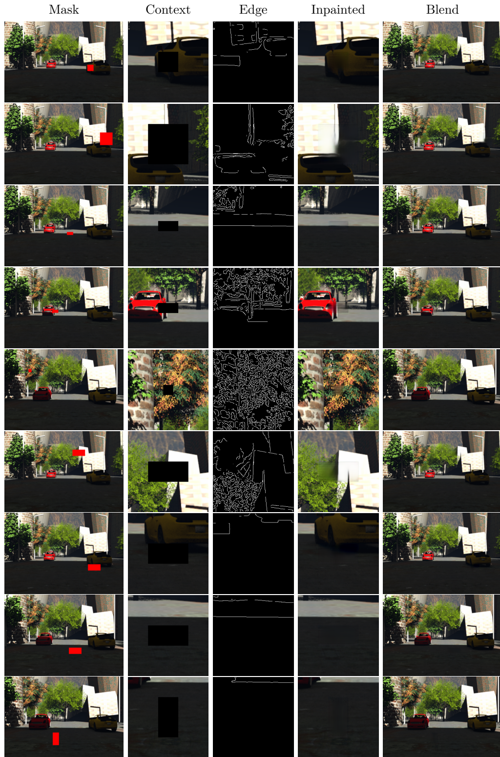
Figure 3.17: Model performance. Mask: Target image with masked synthesis area in red. Context: RGB crop fed into the network. Edge: Edge map fed into the network. Inpainted: our inpainted results. Blend: Target image with our inpainted region. Dataset: Driving [98].
