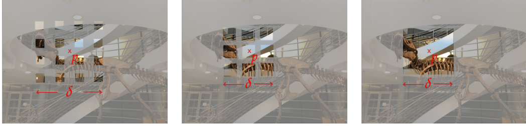
Figure 4.5: Variable patches. An illustration of the varying patch scale over the course of training, which allows the discriminator to learn independently of the image resolution.
