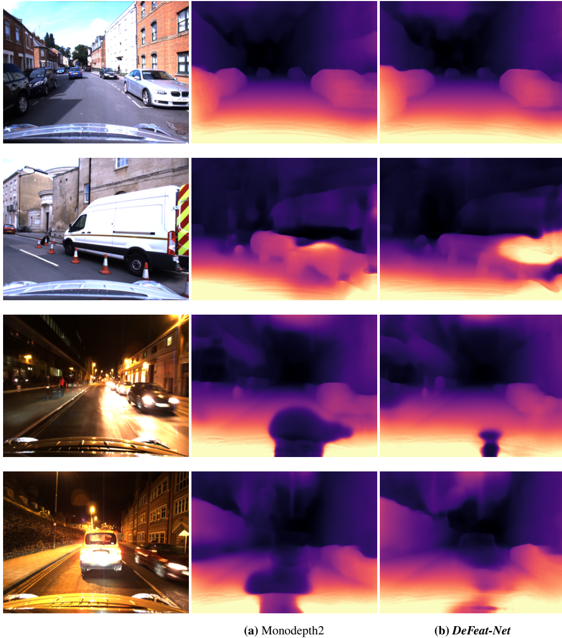
Figure 5.4: RobotCar Depth Estimation. We visualize the network predictions on the RobotCar data. DeFeat-Net provides clear improvements under the challenging night-time conditions. The basic photometric loss is not capable of providing effective supervision in these conditions, leading to more holes of infinite depth.
