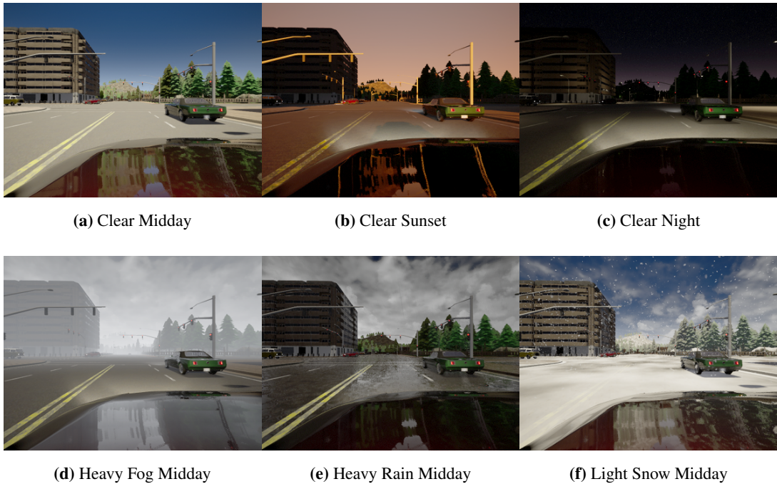
Figure 4.4: CARLA Seasons Sample Images. We show a subset of the 27 total combinations of seasonal and weather effects available in the CARLA Seasons dataset. By making use of simulated environments, perfectly aligned data is provided—including dynamic objects—which is practically impossible to obtain in the real world.
