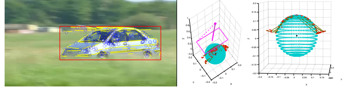
Fig. 9. State of the proposed TMAGIC tracker after the first frame. Left: a bounding box, \mathcal{X}^1 and \mathcal{L}^1 . Right: \mathcal{X} , \mathcal{L} , initial model M (the blue sphere visualises sampled points \mathcal{M} ) and C^1 (magenta). For the camera, the visualisation shows the projection centre C , principal direction and image plane. The upper left corner of the image plane is indicated by the dashed line.
