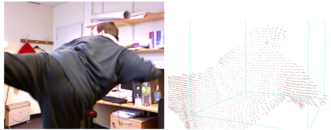
Fig. 1: An estimated 3D motion field, from a sequence of a person performing a kicking action. Motion vectors move from the red to purple vertices.
