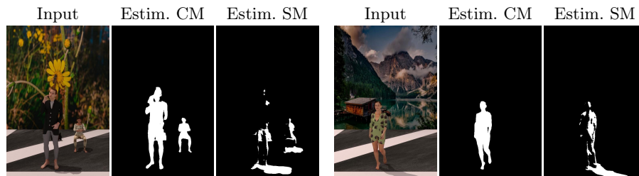
Fig. 3: Examples of RenDetNet’s caster & shadow identification abilities - Dataset #2
