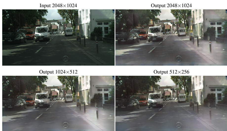
Figure 3: Lighting transfer results for a Cityscapes image re-styled using SILT trained on the Multi Illumination dataset. The numbers next to ‘Output’ show the size of the input image used to create the output image (of the same size).
