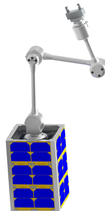
Fig. 1: A space robot is defined as a manipulator of any number of d.o.f. mounted on a base spacecraft of any size.
