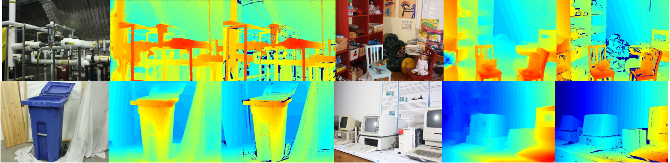
Figure 6: Example Half resolution reconstructions from the Middlebury 2014 dataset. Each triplet shows one input image (left), the output of our algorithm (middle) and the ground truth (right).
