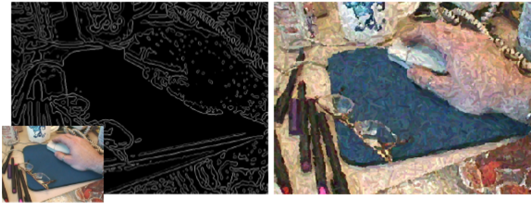
Figure 2-4 Illustrating Litwinowicz’s painterly video technique — images reproduced from [103], original inset. Sobel edges (left) are computed for each frame; strokes are placed and clipped to these edges (right). Strokes are translated over the course of the animation, according to the optical flow vectors computed between frames. This algorithm represents the state of the art in creating automated painterly animations from video.
